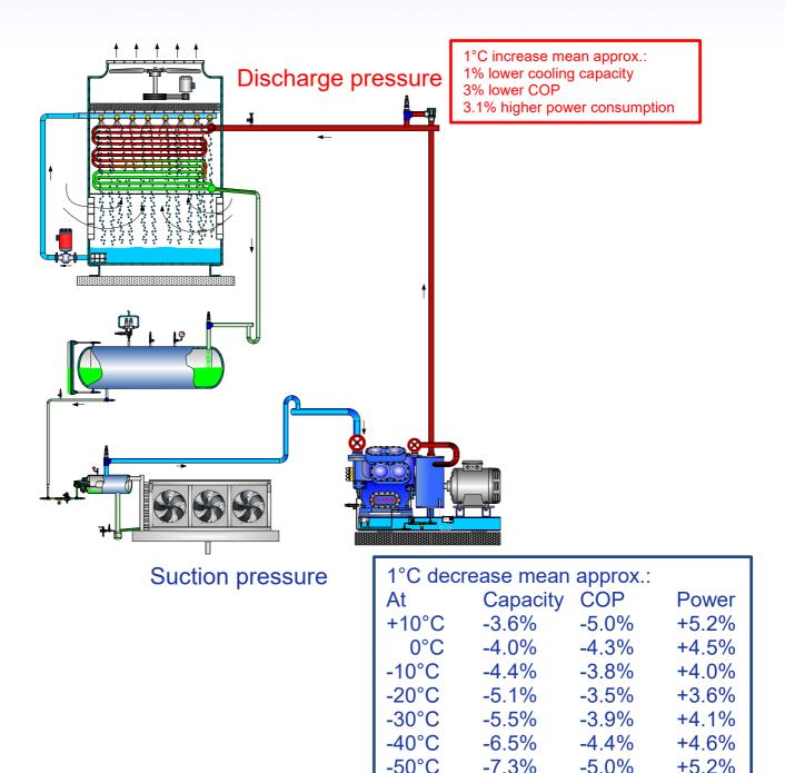
Numbers from average of Sabroe recip and screw Power is with unchanged cooling capacity
