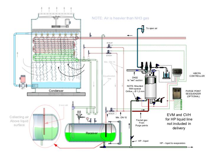
Note ø1.2mm orifice in HP feed line, included on request
