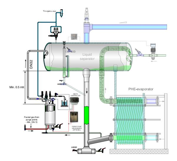
Minimum 0.5m gravity height for self circulation
