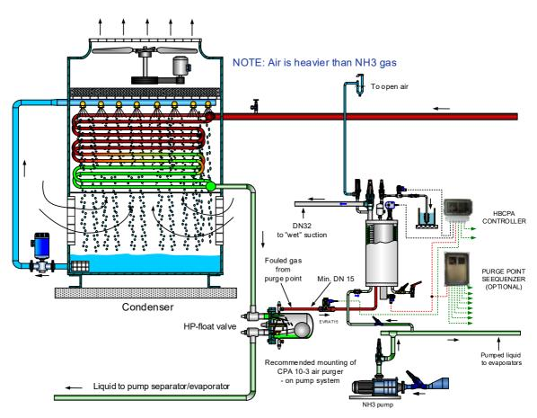
Recommended Purge Point connection to HP float valve Pumped LP liquid feed to CPA
